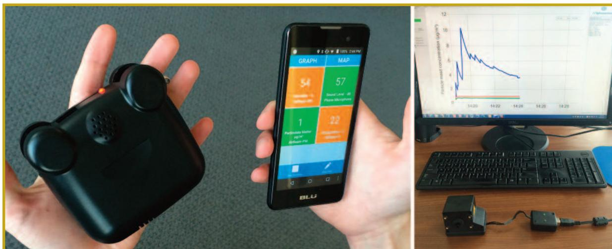
**Figure 2.** The AirBeam system (left) includes a particulate matter sensor, Bluetooth data communications, and the AirCasting app and website for data visualization. The Alphasense OPC (right) is a particulate matter sensor with a hardware-to-computer interface. These are two selected air sensor systems among many available.
